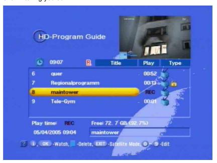
With the buttons, you can select a currently running or previous recording and start the playback by pressing . The recorder plays the recording you selected. "h\*\*\*" appears on the LED display.
